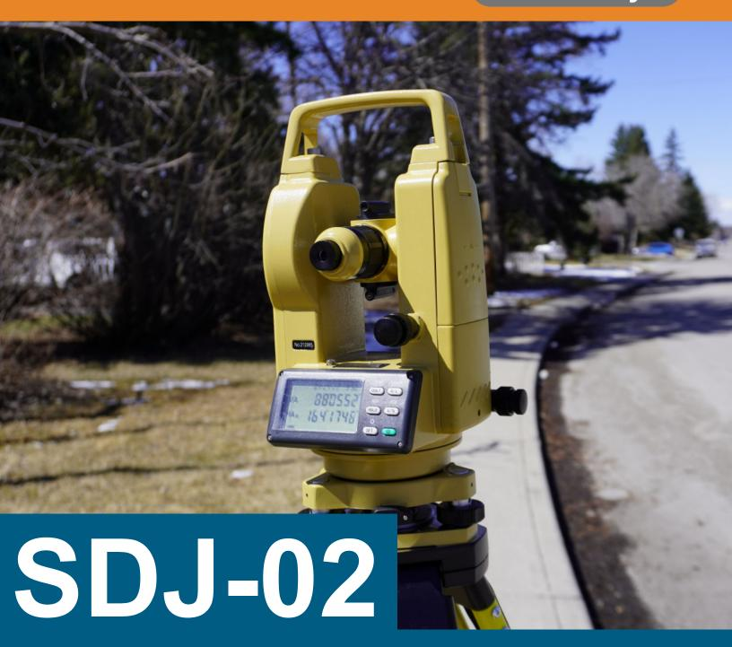
Theodolites is a precision instrument for the measurement of angles in the hoirzontal and vertical plane. They are commonly used in surveying, construction, and engineering for tasks such as measuring the elevation of a structure, determing the slope of a surface, and creating topographic maps.
