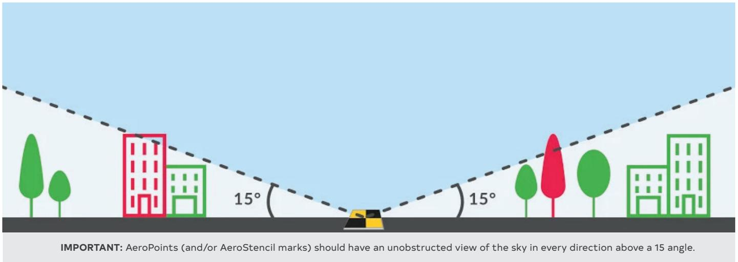
Operators should also avoid placing AeroPoints near buildings or rock faces to minimise the effect of the AeroPoint receiving multiple reflected signals from the same satellite (an effect known as 'multi-pathing').
